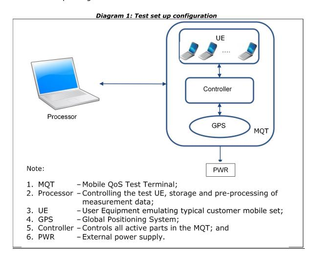
12. The test call number will be a switch terminating number (for inter-network and intra-network testing) i.e. the test will only measure the call setup success rate and dropped call rates of the mobile originated call network.
