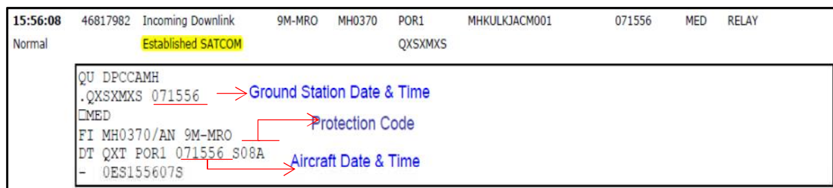
Figure 1.9D: ACARS data link established SATCOM transmission
