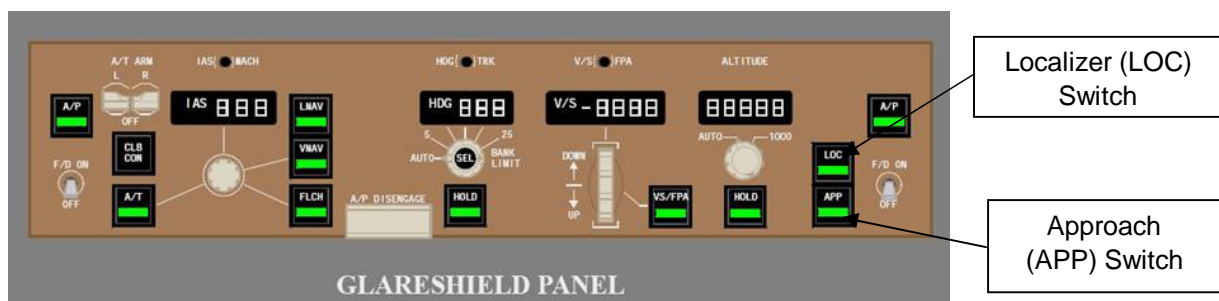
Figure 1.6ED Approach Mode Switches
