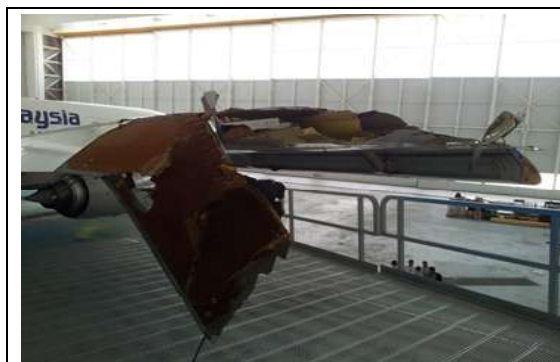
Figure 1.6A - Right Wing Tip Damage
