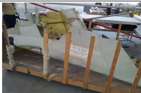
Figure 1.6B – Damaged Wing Tip
