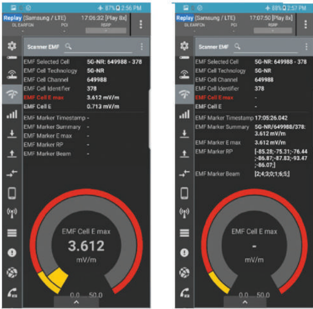
Figure 14: QualiPoc screenshots when searching for the maximum electric field strength in mV/m (left) and marking the cell after the maximum is found (right)
