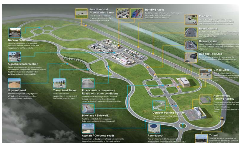
Figure A2.29: Autonomous Vehicle test bed; Source: Korea Automobile Testing & Research Institute (KATRI)
