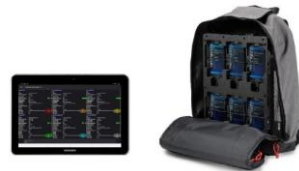
Figure 1: NWA measurement system, which includes one Master unit (tablet) with 6 test phones ( 16 sets nationwide )
