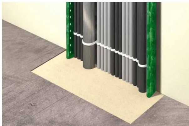
Figure 17. Proper floor hacking
