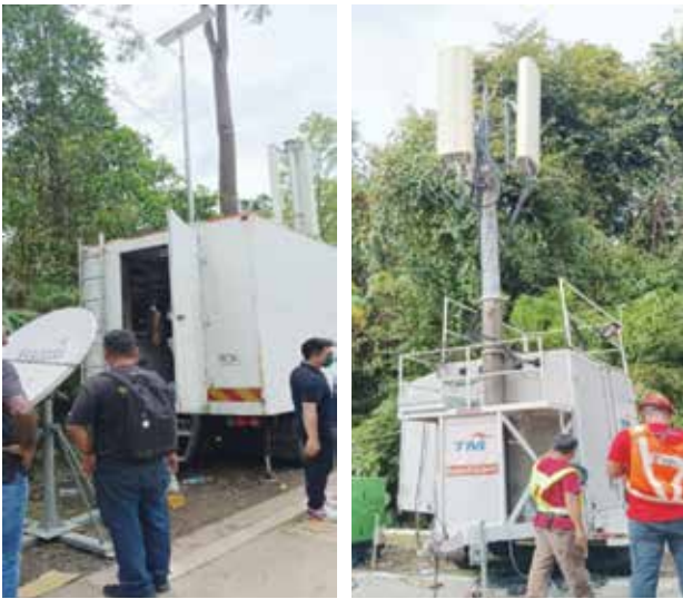
Image 5: Maxis Cell on Wheels (CoW) and TM CoW (Source: MCMC Selangor Database)
