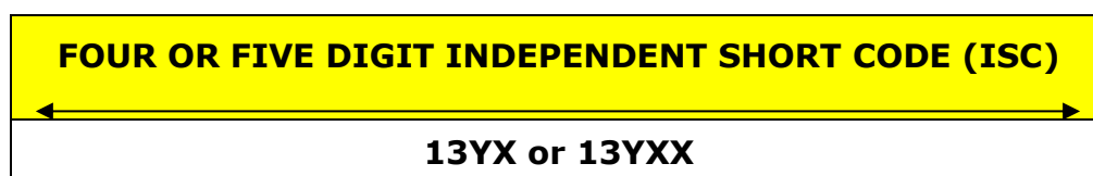
FIGURE 7.3: NUMBER STRUCTURE FOR INDEPENDENT SHORT CODE
