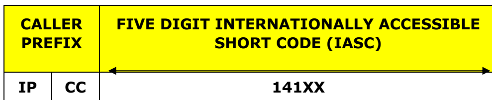
FIGURE 7.4: NUMBER STRUCTURE FOR INTERNATIONALLY ACCESSIBLE SHORT CODE
