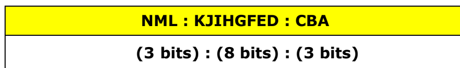
FIGURE 10.8: NATIONAL SIGNALLING POINT CODE FORMAT
